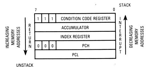
NOTE: Since the Stack Pointer decrements during pushes, the PCL is stacked first followed from the first of the stack is in the reverse order. Go to: www.freescale.com
